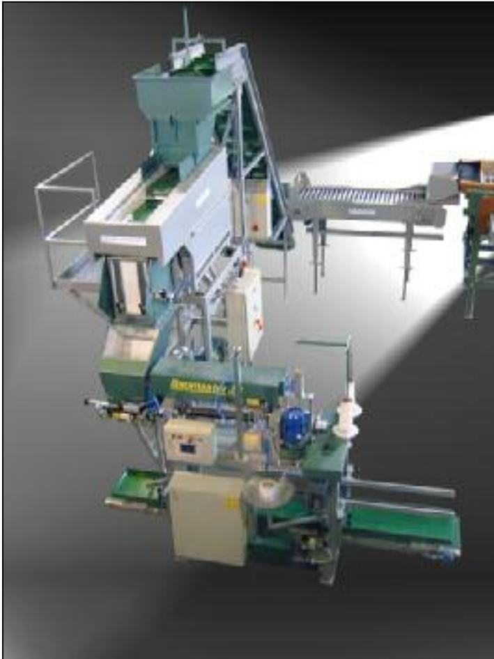
Single Electronic Weigher with bagger JN-ZK1
