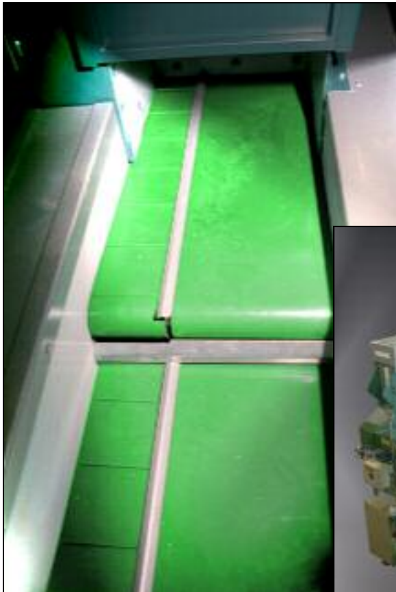
Belts feeding the weighing bucket
